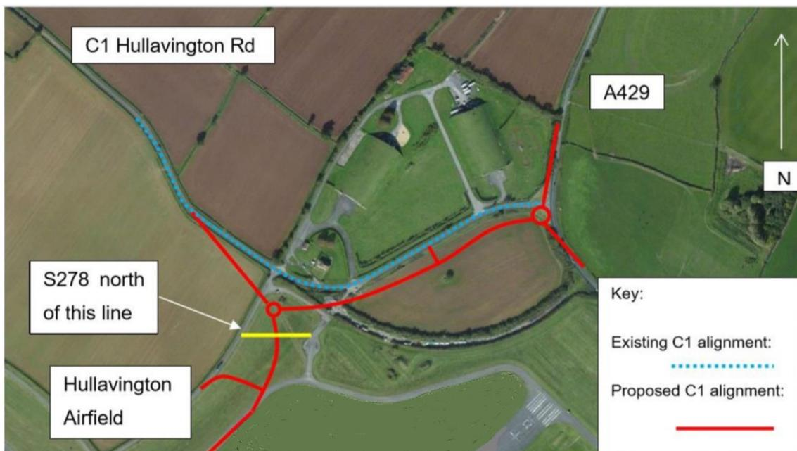
The image shows in red the alignment of the new link road compared to the existing in blue.
